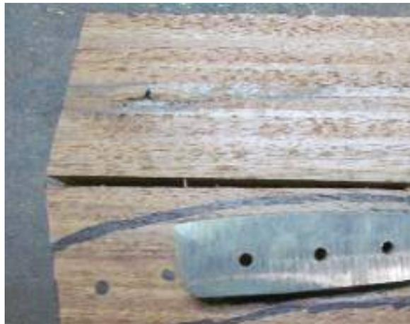
Position the tang on one scale and securely clamp it in place. If the tang has a significant dorsal to ventral taper, you can grind that somewhat flat back of the throat plane. When positioning the blade on the scale, make sure that there is no air gap between the back surface of the recess cut and the front surface of the block. It is better to have the wood surface slightly proud than leaving a gap.
