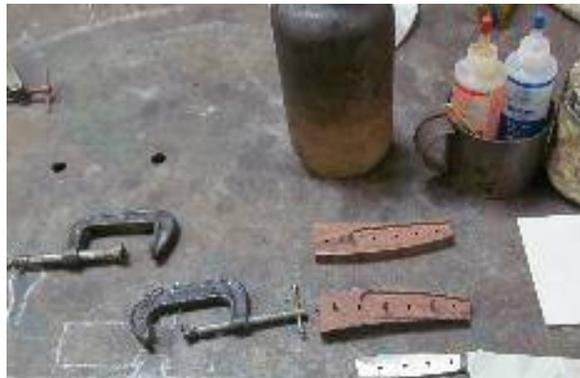
I like to have the center clamp on the opposite side of the handle from the other two clamps. Remove and wipe off the pins. Use a paper towel wetted with acetone and wipe off the throat area. Wait until the epoxy sets.
