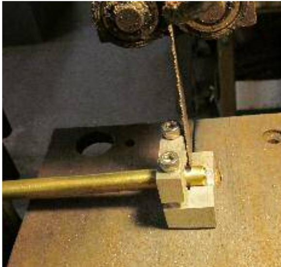
Gently insert a pin into the handle - just enough so it doesn't fall out. Flip the handle over and do the same for the other pin. A block of wood with a hole larger than any pin stock you use makes a convenient way not to mess up one side while working on the other.
