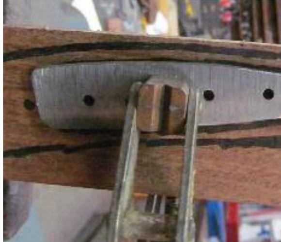
Since the scale is flat, a wood block can be used to create a horizontal plane over the drill press vise. A relatively narrow block (0.5"-.0.75") is convenient and minimizes the number of times you have to reclamp. If you reclamp, be sure to use temporary pins and/or set another clamp before moving the first clamp. The tang cannot move relative to the scale. Drill the holes using the tang as a template.
