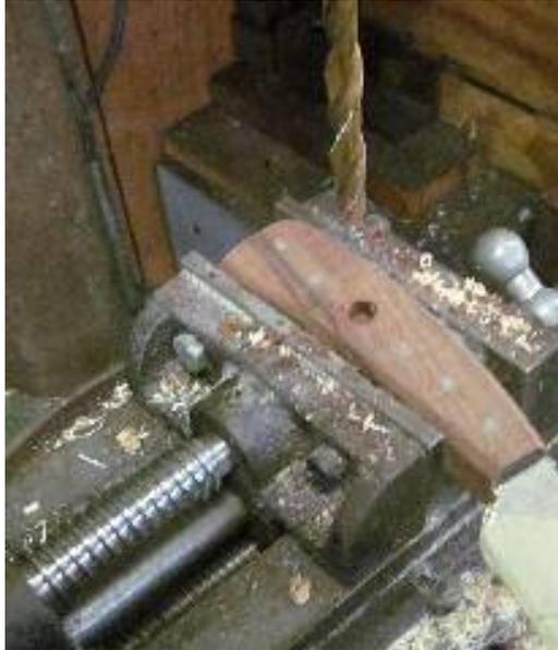
Use the depth gauge and determine the maximum depth you drilled. Lay out the distance on the pin stock (which should have beveled ends). Use the saw tool and cut off the two sections needed. Bevel-grind the ends of the remaining stock for next time.
