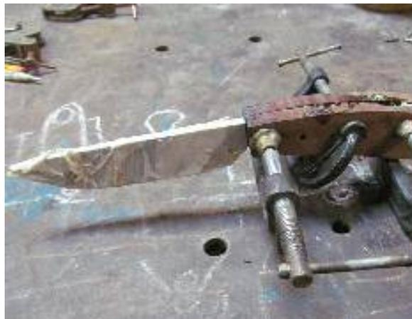
Grind off the epoxy splatter so that the handle will lay flat when drilling. Drill out the pin holes - if using undersized bits, now use 1/8" bit to match pin stock. Layout the length of pins needed - deliberately oversize them - wasting an 1/8" or .a 1/4" of stock is far better than coming up short. If using a mosaic pin, make n-1 pins where n is the number of holes.
