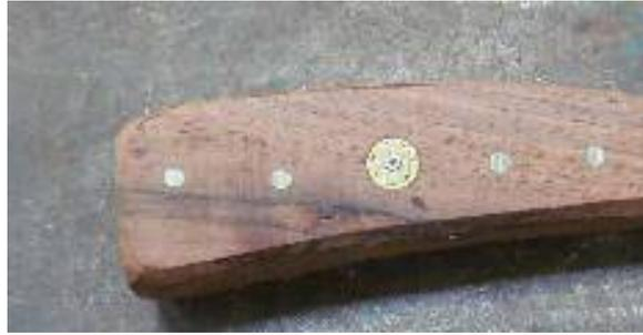
Buff with white rouge. Remove the tape and sharpen the blade. For a patterned blade, you can use gun bluing and a wet 2000 grit sandpaper to pop the pattern. Dry and then apply hot beeswax to finish.
